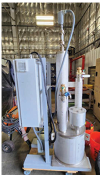
Figure 2. 7 kW heater used to test the hydrogen target loads.
